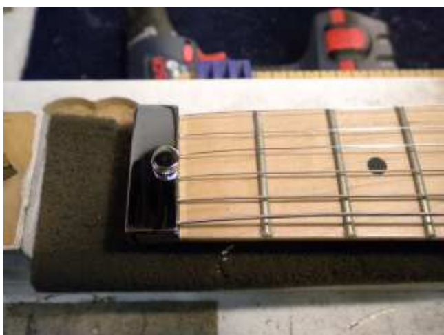
After tuning the strings can be clipped and string cap replaced. The instrument is ready to be played.
